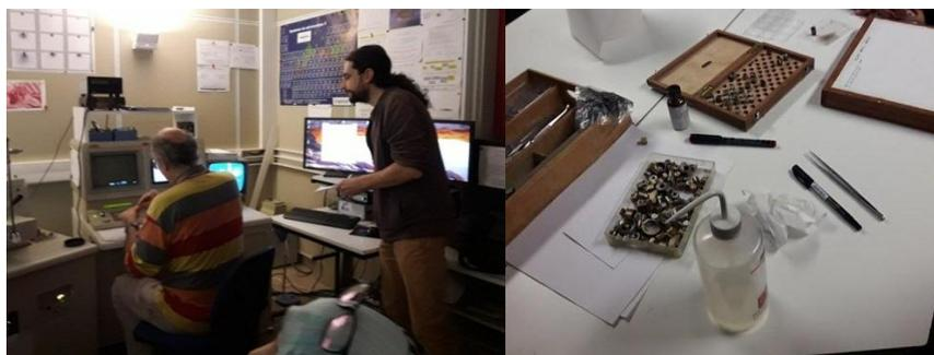
Figure 11 : scanning electron microscope (SEM) (left) and sample preparation for metalization method (right).
