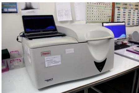
Figure 12: EDXRF instrument at AIGS Laboratory
