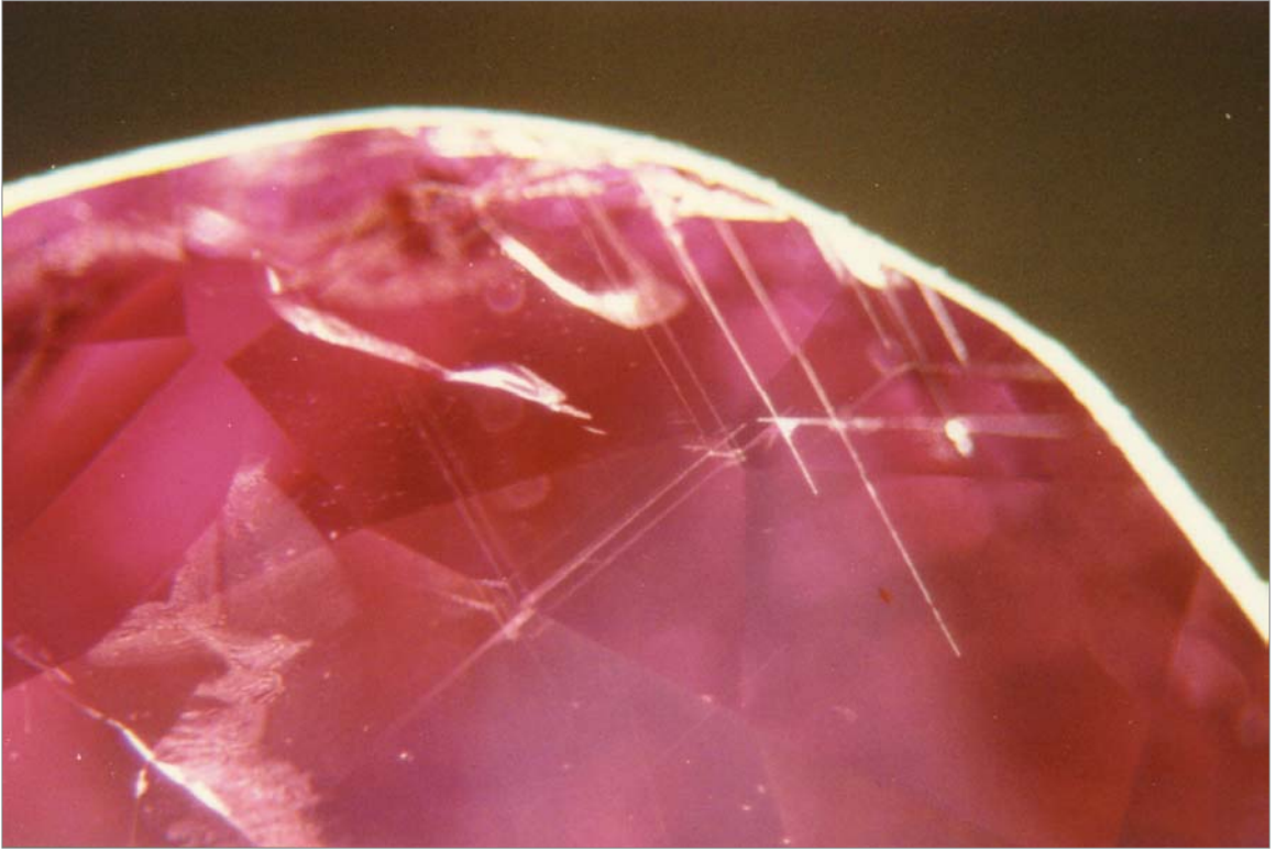
Figure 37. Scaffold of coarse needles of presumably boehmite intersecting in three directions (similar to those encountered in Thai rubies), here observed in (A-04), a pear-shaped ruby of 1.42 ct, from Colombia. Note the dense nest of minute inclusions (unidentified, but presumably rutile). (Dark field illumination 40x)
