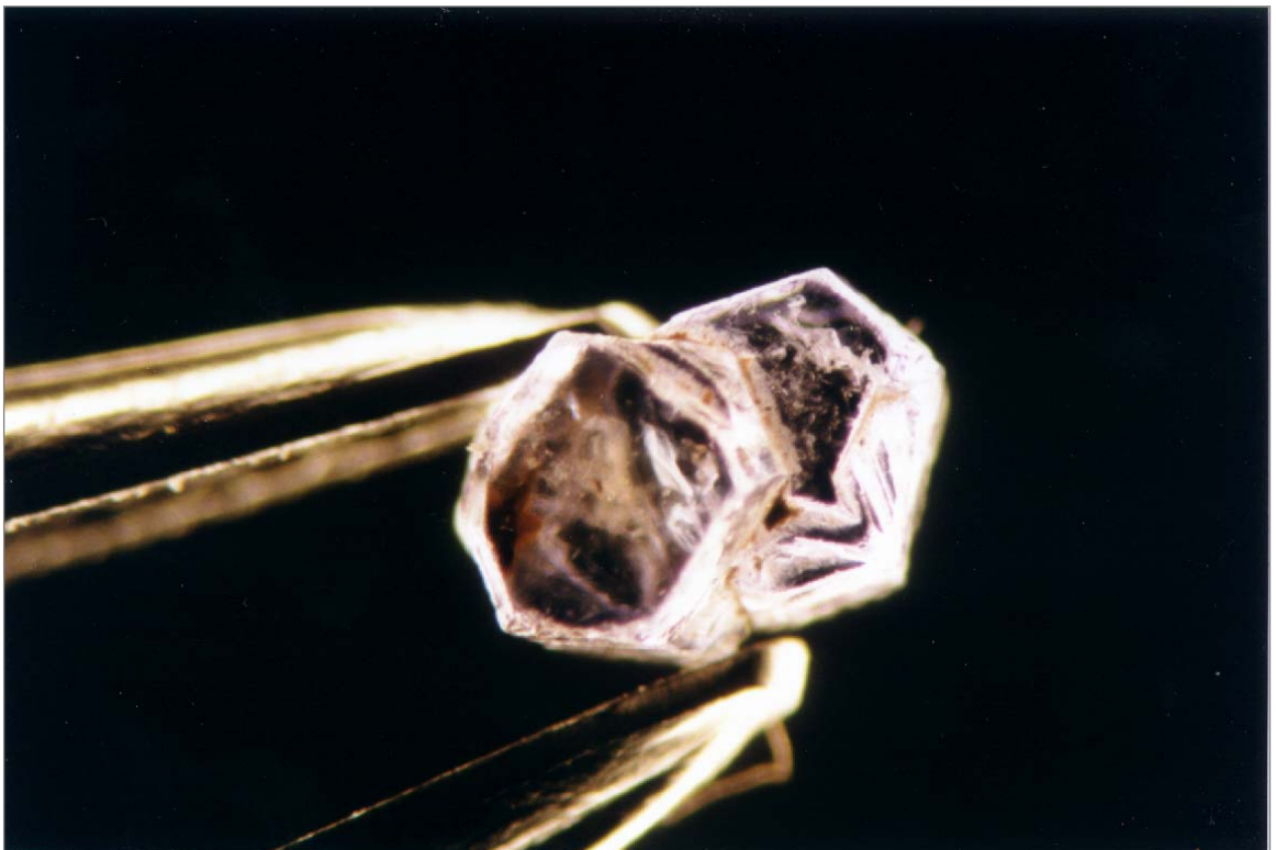
Figure 14. An hexagonal rough sapphire from Colombia, showing interpenetrant twinning very similar to those encountered in rough sapphires from Madagascar. (Dark field illumination 30x)
