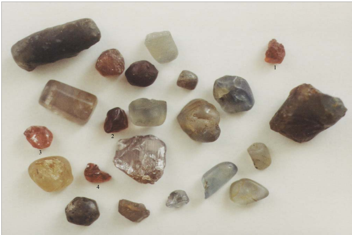
Figure 11. The twenty-two rough crystals from Colombia examined for this study in 1991. The four red crystals were positively identified as garnets by their absorption spectrum. (Size range: 3.30 x 3.30 x 2.50 mm to 6.80 x 6.30 x 16.20 mm)
