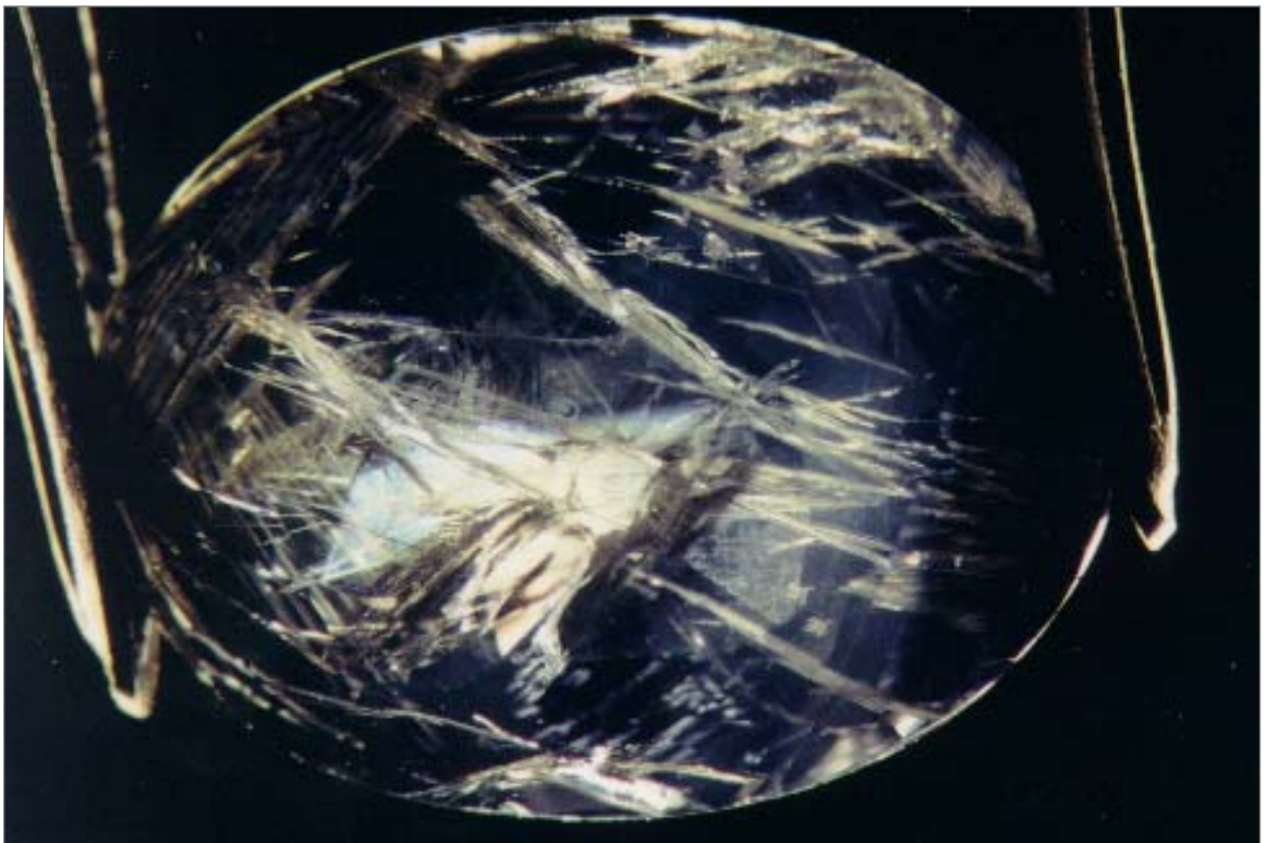
Figure 68. Numerous internal stress fractures, similar in appearance to those caused by “quench-crackling”, were observed in (HH-01), a greyish-blue sapphire of 4.81 ct, from Colombia. (Dark field illumination 20x)
