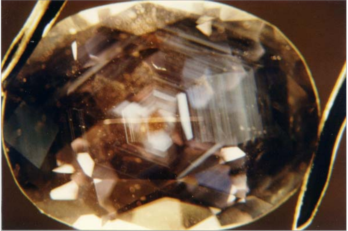
Figure 65. Distinct hexagonal growth steps reminiscent of terraced farmlands (similar to those seen in sapphires from Montana, N. America), observed perpendicular to the C-axis in (A-12), an oval-shape sapphire of 6.89 ct, from Colombia. (Dark field illumination 15 x)
