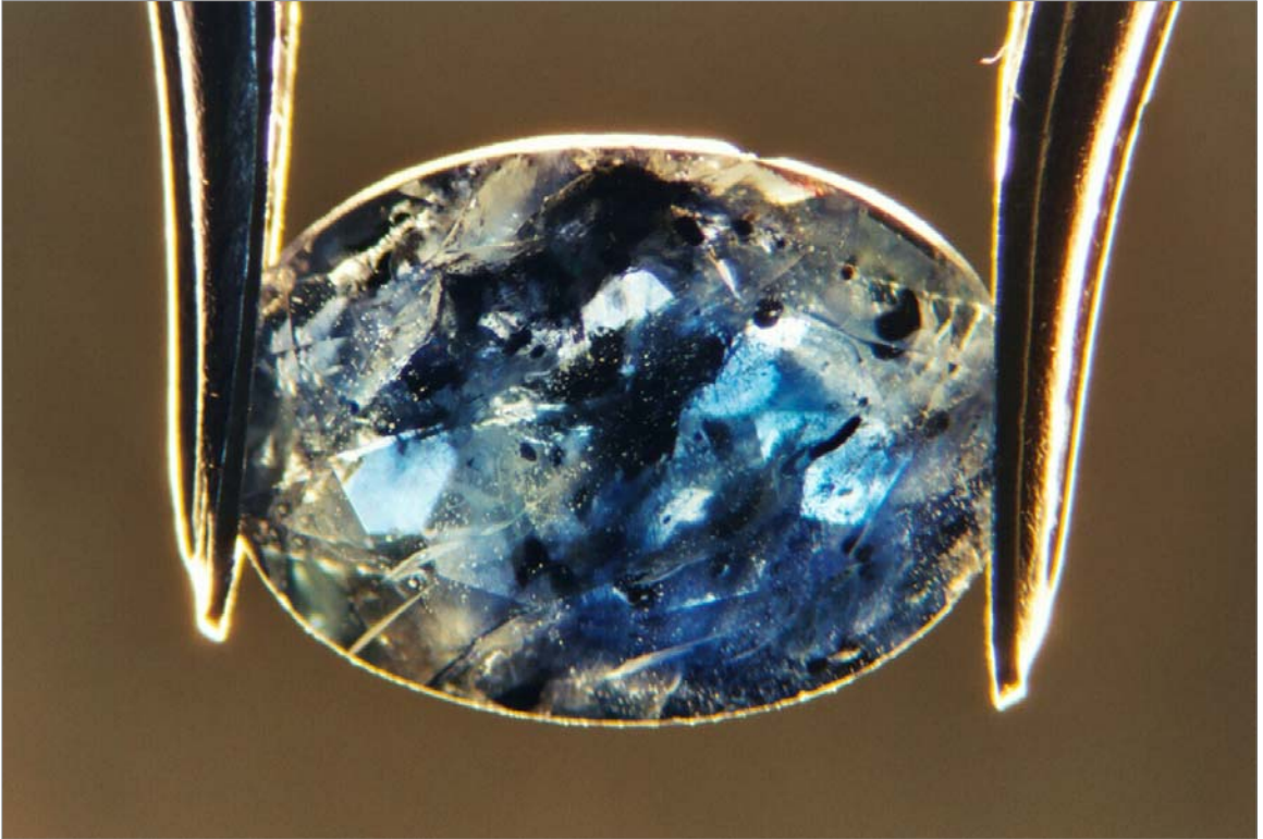
Figure 71. Corroded rutile crystals due to intense heating, diffusing intense blue patches, responsible for the internal dark blue colour of the sapphire. Observed in (TT-01), an oval-shape heat-treated sapphire of 2.14 ct, from Colombia. (Dark field illumination 10x)
