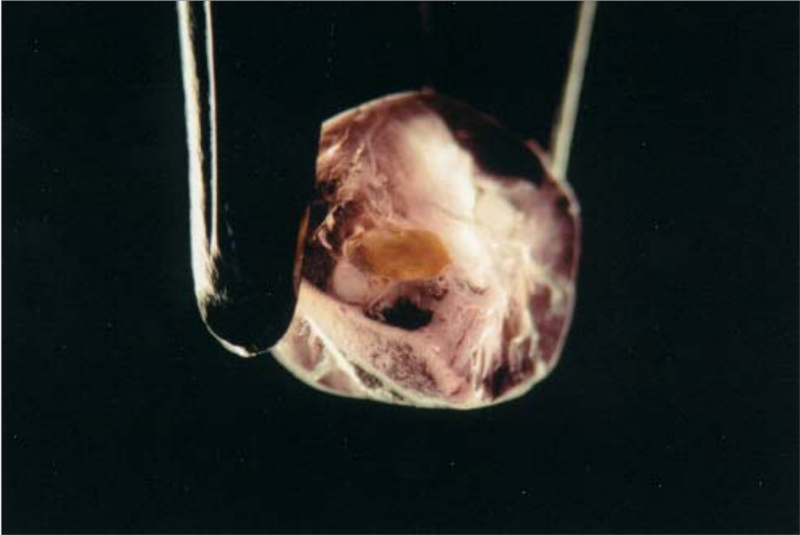
Figure 20. A very small yellow transparent slightly waterworn corundum crystal, partly inside and partly outside in open air, included in a small rounded tabular hexagonal rough sapphire from Colombia. (Dark field illumination 20x)
