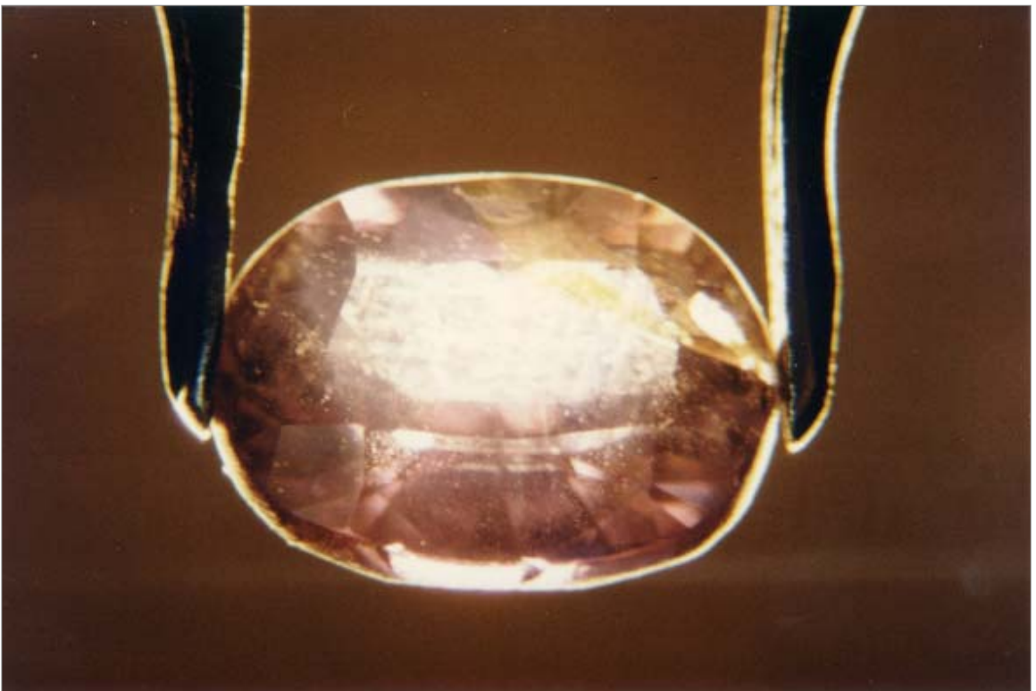
Figure 42. Yellow colour zone observed in (A-02), an oval-shaped ruby of 2.33 ct, from Colombia. (Dark field illumination 10x)
