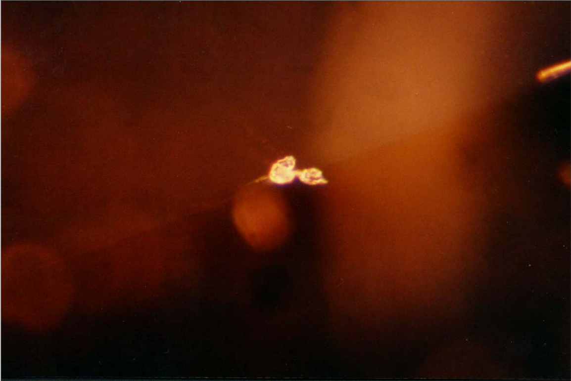
Figure 49. A pair of colourless zircon crystals surrounded by tension fissures (similar to those encountered in sapphires from Sri Lanka), observed in (A-25), a multicoloured oval-shape sapphire of 2.58 ct, from Colombia. (Dark field illumination 80x)
