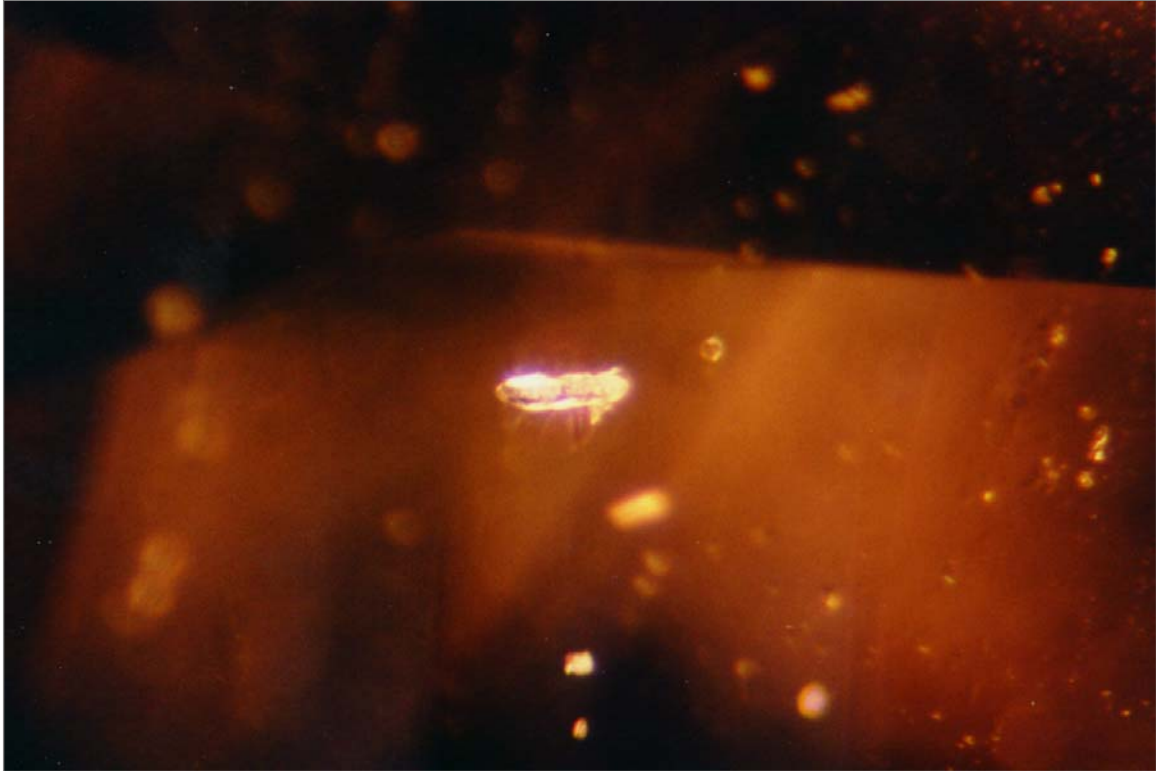
Figure 51. A large doubly terminated colourless zircon crystal surrounded by numerous sets of halos and tension fissures. Observed in the same multicoloured oval-shaped sapphire of 2.58 ct (A-25), from Colombia. (Dark field illumination 80x)
