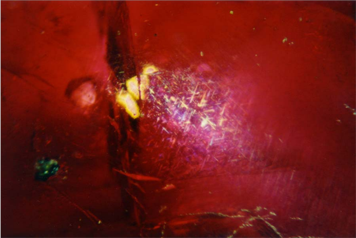
Figure 39. A small dense nest of very short exsolved rutile needles, viewed along the C-axis (similar inclusions are encountered in Myanmar rubies), here observed in (A-06), a cabochon ruby of 1.66 ct, from Colombia. This stone also showed pronounced “bleeding of colour” which is frequently seen in rubies from Myanmar. (Overhead and dark field illumination 45x)
