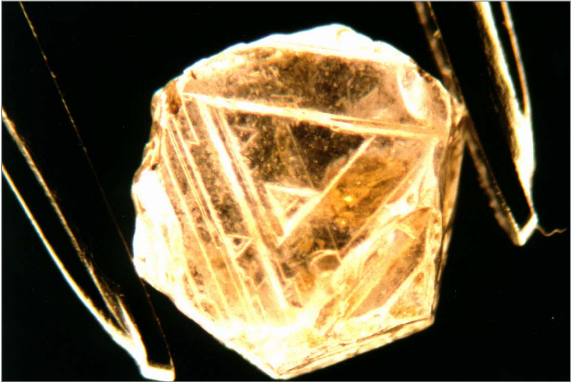
Figure 13. A rough corundum crystal from Colombia, showing a hexagonal prism habitus with triangular growth planes along a basal plane. (Dark field illumination 15x)
