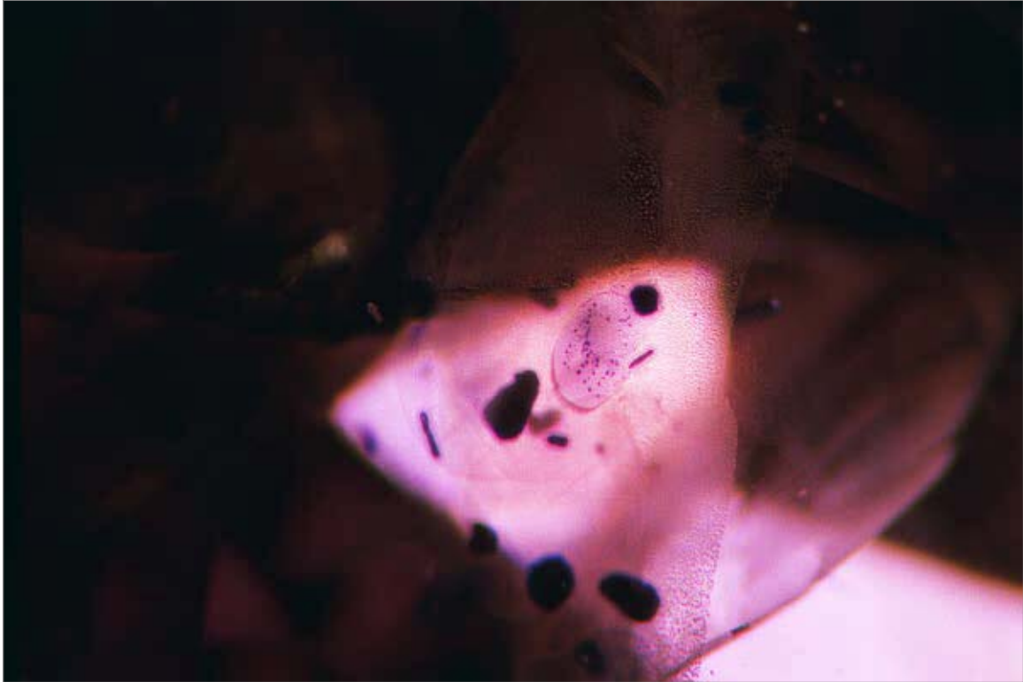
Figure 75. Corroded rutile crystals surrounded by a violetish red halo (incandescent light) containing pinpoint inclusions, observed in (TT-02), an oval-shape heat-treated colour-change sapphire of 0.96 ct, from Colombia. (Dark field and incandescent illumination 40x)
