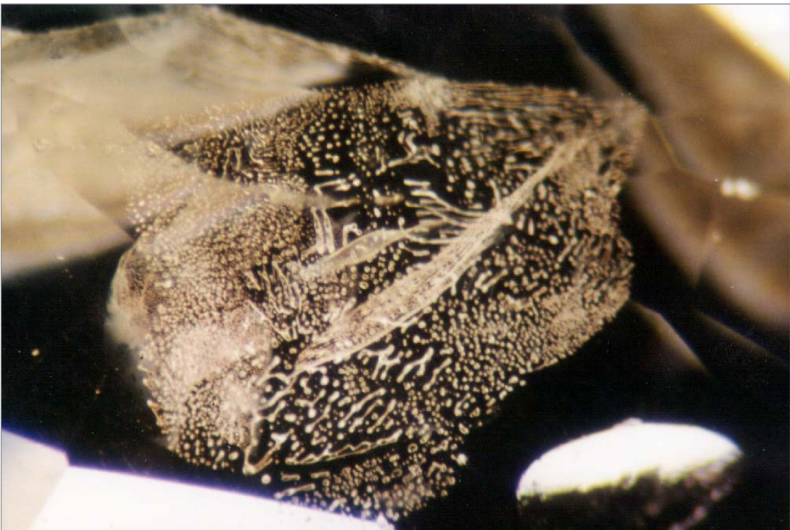
Figure 70. A "fingerprint" filled with two-phase inclusions observed in (A-33), an oval-shape colour-change sapphire of 0.65 ct, from Colombia. (Dark field illumination 40x)
