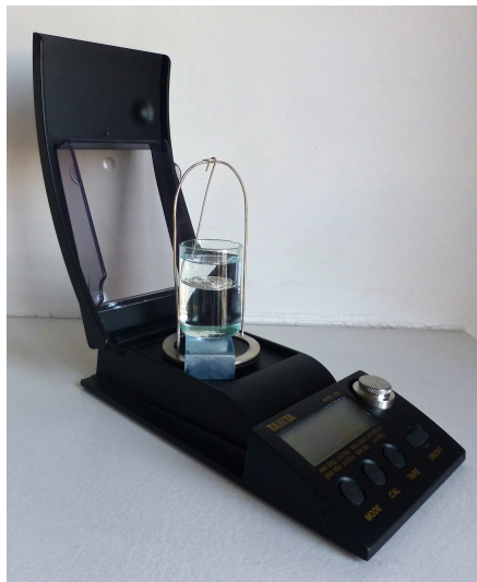
Figure 3 – " Balance hydrostatique ", de fabrication artisanale
