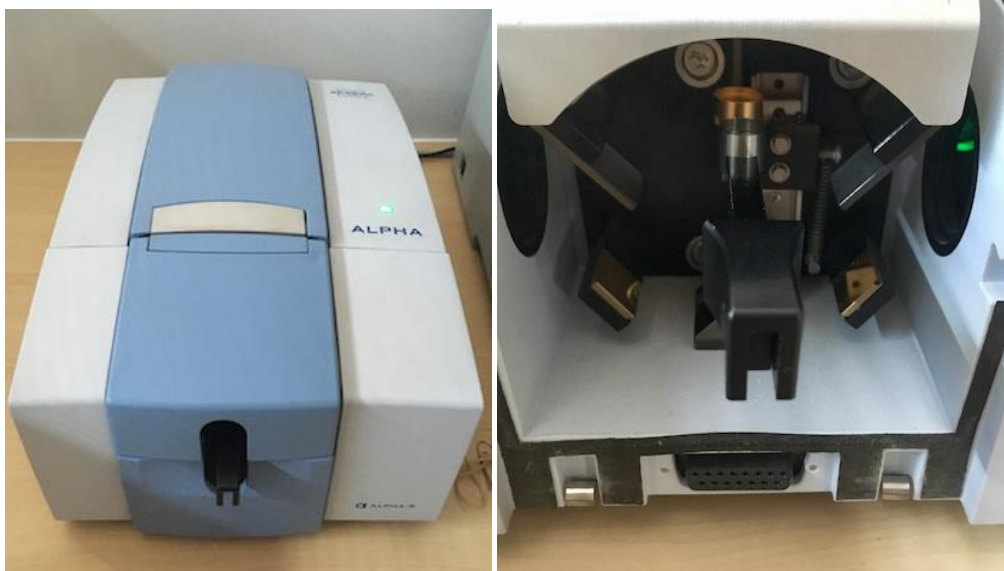
Pic. 4 and 5: Bruker Alpha FTIR with diffuse reflectance attachment. EGL South Africa. Photo: Alix van der Wat
