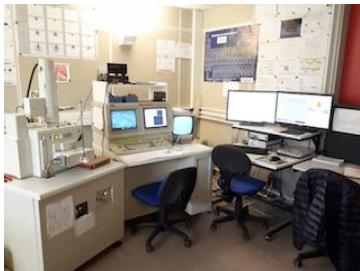
Pic. 1: SEM JEOL 5800LV, University of Nantes. Photo: Pauline Goots
