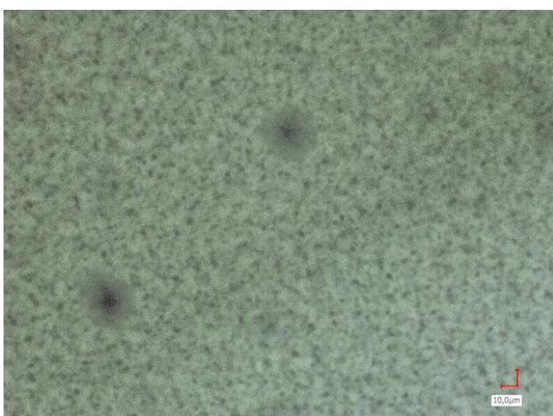
Pic 11 and 12 : LEFT , sample 1288, cloud on cuboid sector. Digital microscope, High Dynamic Range (HDR), magnification x500. RIGHT , sample 1288, cloud. Digital microscope, HDR, magnification x1000.
