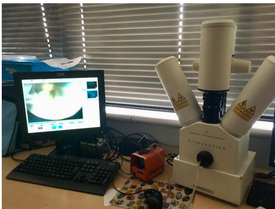
Pic. 2: DTC DiamondView model number 3616, EGL South Africa. Photo: Alix van der Wat
