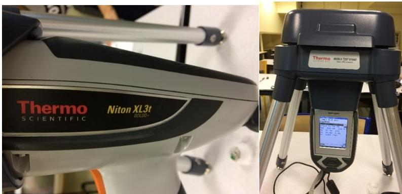
Figure 58 XRF transportable Thermoscientifique Niton XL 3t Gold +
