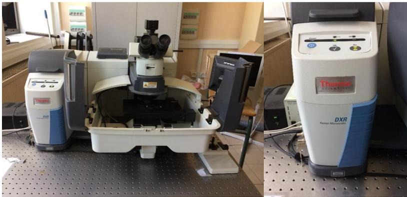
Figure 46 : Raman DXR 780 nm Thermoscientific microscope, Olympus TH4 200.
