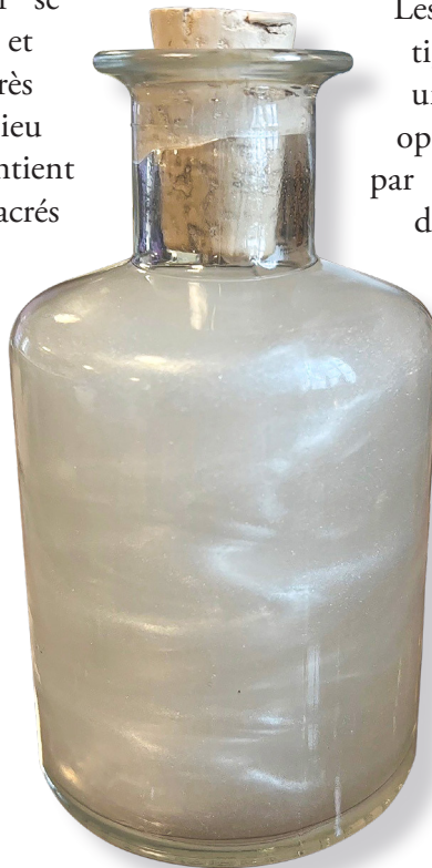
Figure 7: Appearance of the alcoholic solution of crushed fish scales. At rest, the solution will be clear and transparent, after sedimentation of all fine particles at the base of the flask. Photo: Romain Gauthier.
