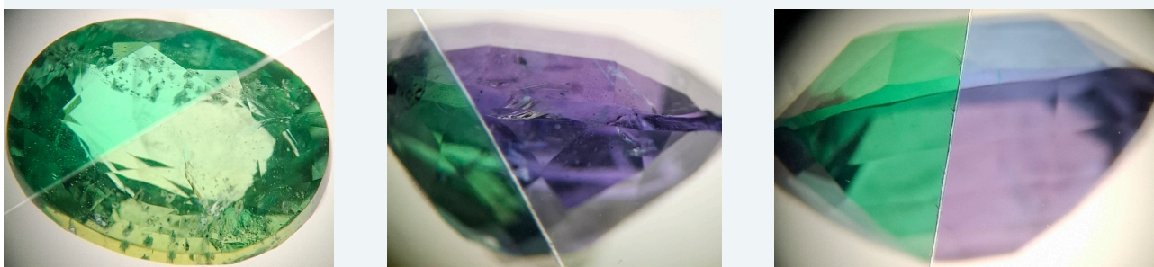
Fig. 5 Examples of pleochroism in KTJ2, KTM and KUF. Observed under stereo microscope with a dichroscope. From left to right: 9.52x7.40mm, 8.98 x 7.03mm and 9.71 x 8.31mm.
